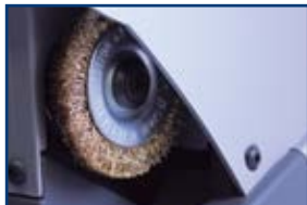
6 Brush for deburring the key. Brush protective area.
